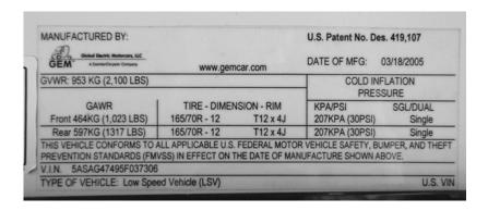
Manufacture Sticker located on underside of roof. The Date of Manufacture is listed on upper right hand corner
